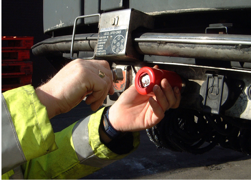
Castell Salvo locked in place on a trailer's emergency air line
